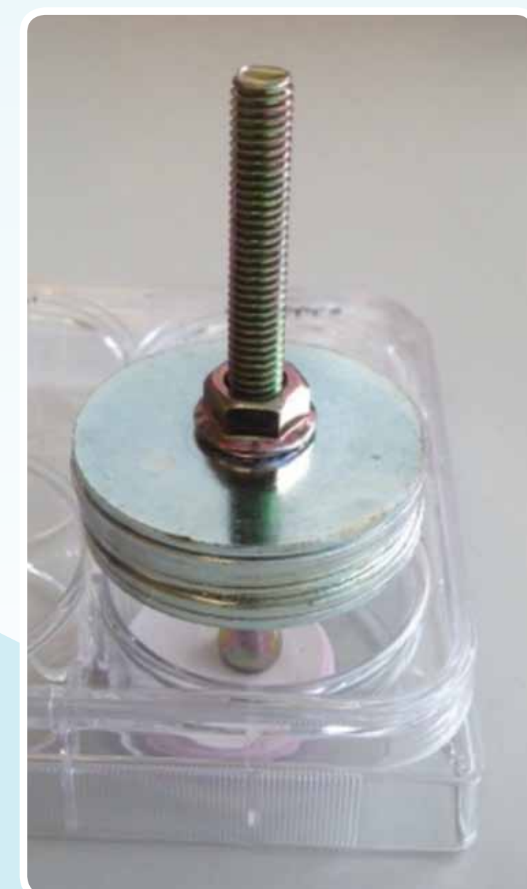
Figure 2 Custom-built loading device used to apply sustained pressures (Bronneberg et al, 2007)
