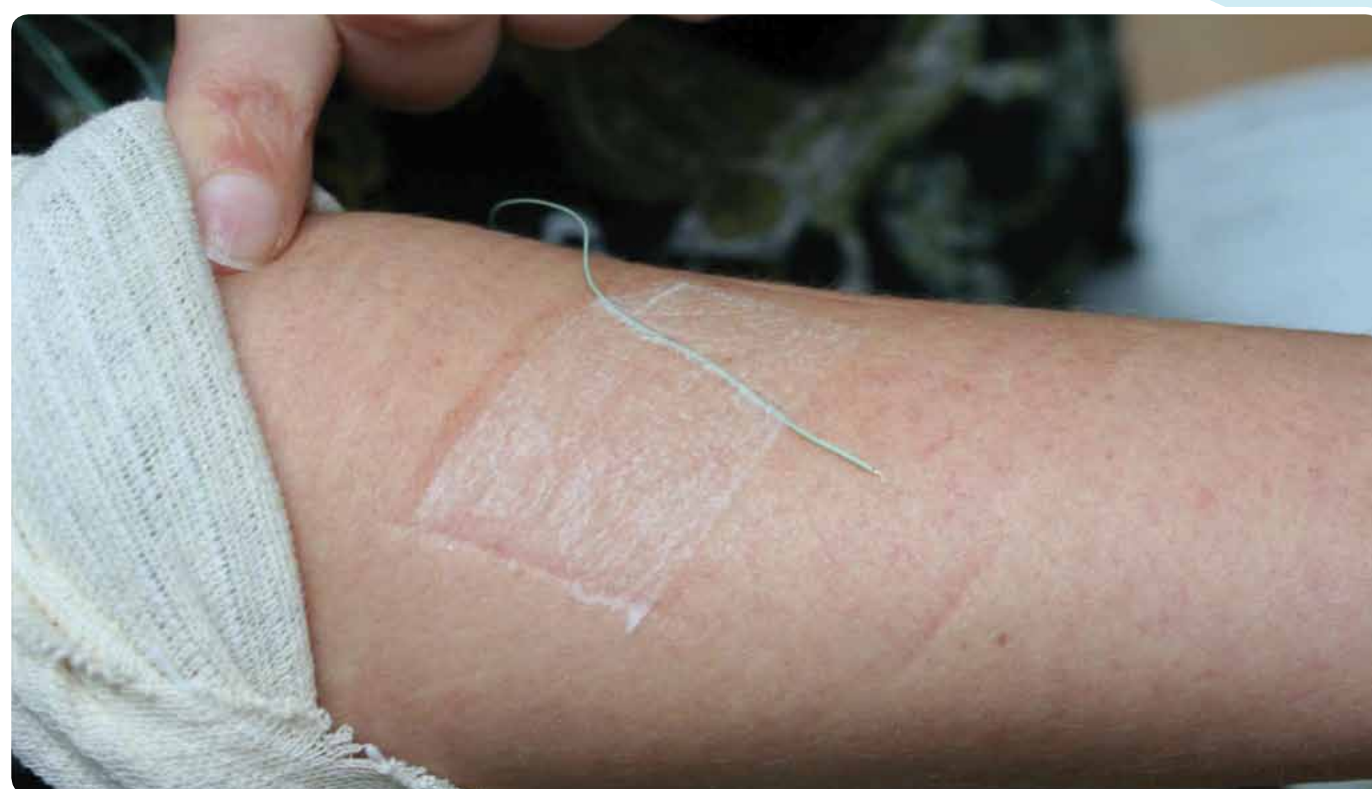
Figure 1 Thermocouple probe placement
